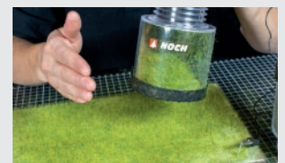
The change enables 'flocking' with different grass fibres before the adhesive dries.
