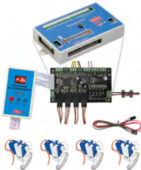
47PLS100 (PLS100) SmartSwitch Starter-Set Contents • SmartSwitch Control Board • Programming Board • 4 x servos • 4 x switches • 4 x operating wires
