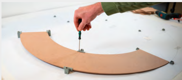
The Basic Helix is assembled directly on the enclosed plan. The base plates are fastened to the base plate with screws.
